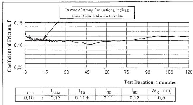
FIG. X1.1 Example: Recording and Evaluation of Friction Coefficients
